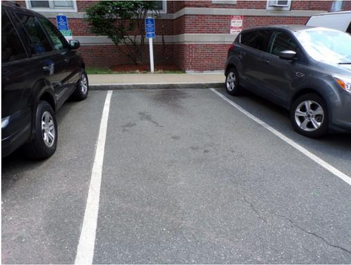
Apartment building 1 handicap parking no pavement markings or access aisle (Critical Repair)
